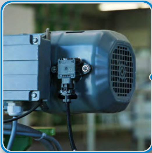
DATAEAGLE Condition Monitoring System (CMS) sensor mounted on motor
